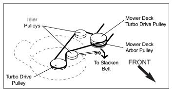
Figure 18. Turbo Belt Routing
